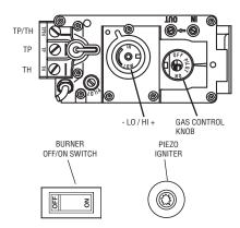
Note: Knob cannot be turned from "PILOT" to "OFF" unless the knob is pushed in slightly. Do not force.
